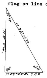
flag on line on right bank; then measure a base on sand bar N. 89° 54' E., 7.70 chs. dist. to a point from which a flag bears N. 26° 33' W.; from flag, E. end of base bears S. 26° 33' E.; therefore, the dist. is cot. 26° 27' x base, or 2.0101 x 7.70 chs. = 15.48 chs., and 14.55 + 15.48 is
