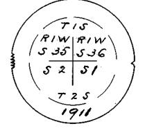
of sees. 1, 2, 35 and 36, marked as in this diagram; dig pits, 18 x 18 x 12 ins., in each sec. 5½ ft. dist.; and raise a mound of earth, 4 ft. base, 2 ft. high, W. of cor.
