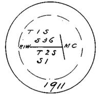
cor. of frac. secs. 1 and 36, marked as shown in this diagram; dig pit, 36 x 36 x 12 ins., W. of cor. 8 ft. dist.; and raise a mound of earth, 4 ft. base, 2 ft. high, W. of cor.; from which
