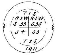
sees. 3, 4, 33 and 34, marked as in this diagram; dig pits, 18 x 18 x 12 ins., in each sec.  $5\frac{1}{3}$  ft. dist.; and raise a mound of earth, 4 ft. base, 2 ft. high, 3. of eor. Chains. Land, level, Harsny; covered with light layer of moss. Soil, sandy; 3rd rate. No timber; dense birch brush.
