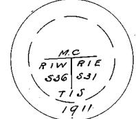
gram; dig pit, 36 x 36 x 12 ins., S. of cor., 8 ft. dist.; and raise a mound of earth, 4 ft. base, 2 ft. high, S. of cor; from which
