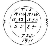
secs. 4, 5, 32 and 33, marked as shown in this diagram; dig pits 18 x 18 x 12 ins., in each sec. 5% ft. dist.; and raise a mound of earth, 4 ft. base, 2 ft. high, W. of cor.
