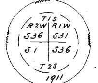
dig pits, 24 x 24 x 12 ins. on each linc. N., E., V., 4 ft., and S. of pipe, 8 ft. dist.; and raise a mound of earth, 5 ft. base, 2½ ft. high, S. of cor.
