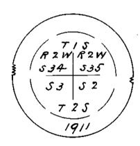
dig pits, 18 x 18 x 12 ins., in each sec. 5% ft. dist.; and raise a mound of earth, 4 ft. base, 2 ft. high, W. of cor., from which A spruce, 5 ins. diam., bears S. 1º 30' W., 47 1ks. dist., mark-
