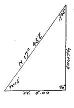
bears N. 17° 45' E.; from F.C. the W. end of base bears 5. 17° 45' W.; therefore, the dist. is cot. 17° 45' x base, or 3.1240 x 5.00 = 15.62 chs. I measure back 1.31 chs., and 15.62 + 8.99 -1.31 is
