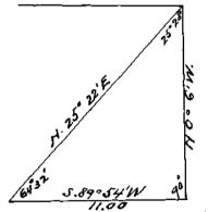
across channel, on a second sand bar; then neasure a base S. 89° 54' W., 11.00 chs. dist., to a point from which flag bears N. 25° 22' E.; the W, end of base, bears S. 25° 22' W. from flag; therefore, the dist. is cot. 25° 28' x base, or 2.0997 x 11.00 = 23.09
