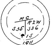
cor. of frac. secs. 35 and 36, marked as shown in this diagram; díg pit, 36 x 36 x 12 ins., 8 ft. S. of cor.; and raise a mound of earth, 4 ft. base, 2 ft. high, S. of cor.
