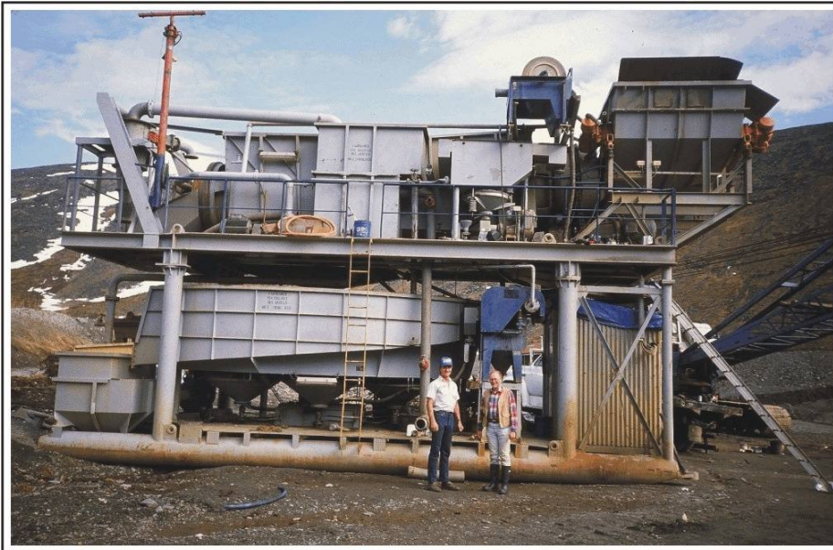
Figure 55. Del Ackels and Odin Strandberg, Jr. standing in front of Ackels' IHC dry-land jig plant on Tobin Creek, June 9, 1990. This equipment was freighted over the Coldfoot-Chandalar Trail during the winter of 1990-1991. Eskil Anderson Collection, courtesy of Richard Walters, LSGMC, Spokane.
