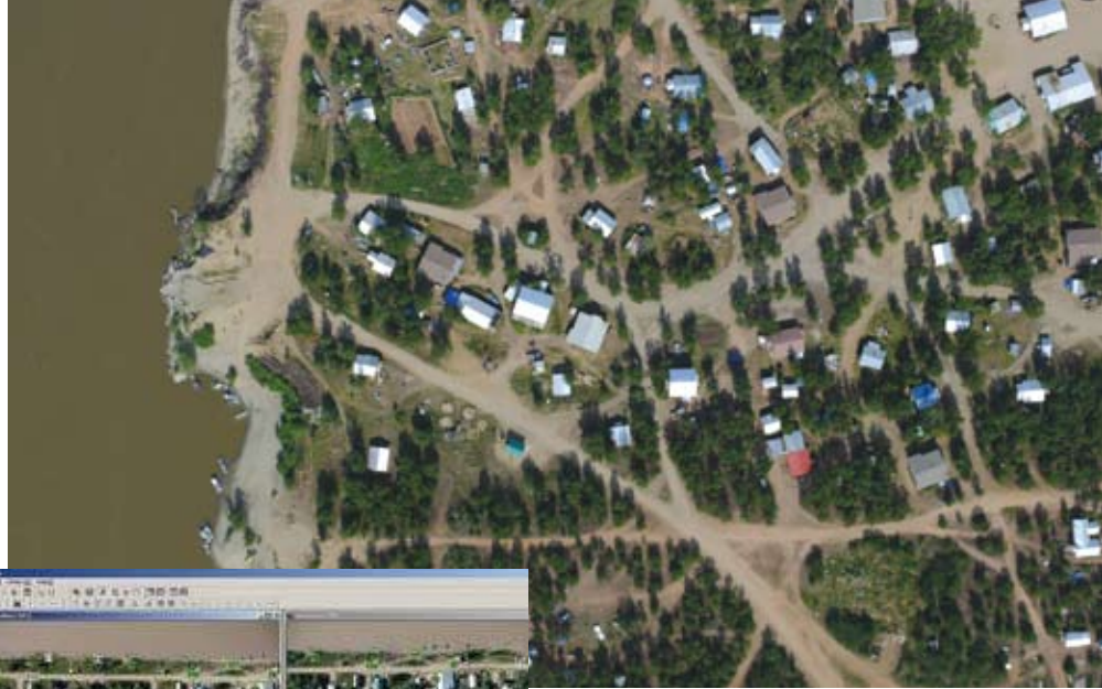
Above: A raw image taken by the Lumix DMC FZ50 that shows complex road patterns in the unsurveyed village of Huslia. Left: This Topcon PI-3000 software screenshot depicts the measurement of control and tie points of a registered stereo pair.
