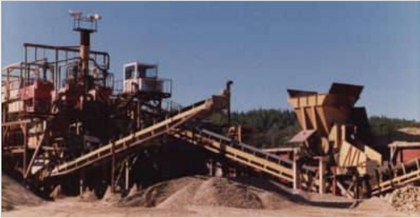
Gold plant control cab with hopper feed conveyor for raw gravel and one of four adjacent discharge conveyors. Photos courtesy of Alice Ellingson
