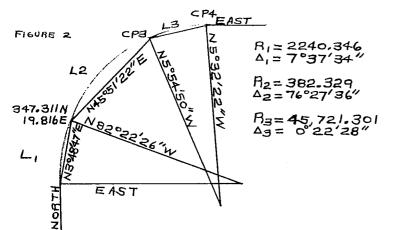
Notice how after the "bump" the compound curve changes. In a more extreme case, an undesired point of reverse curvature could be created.
