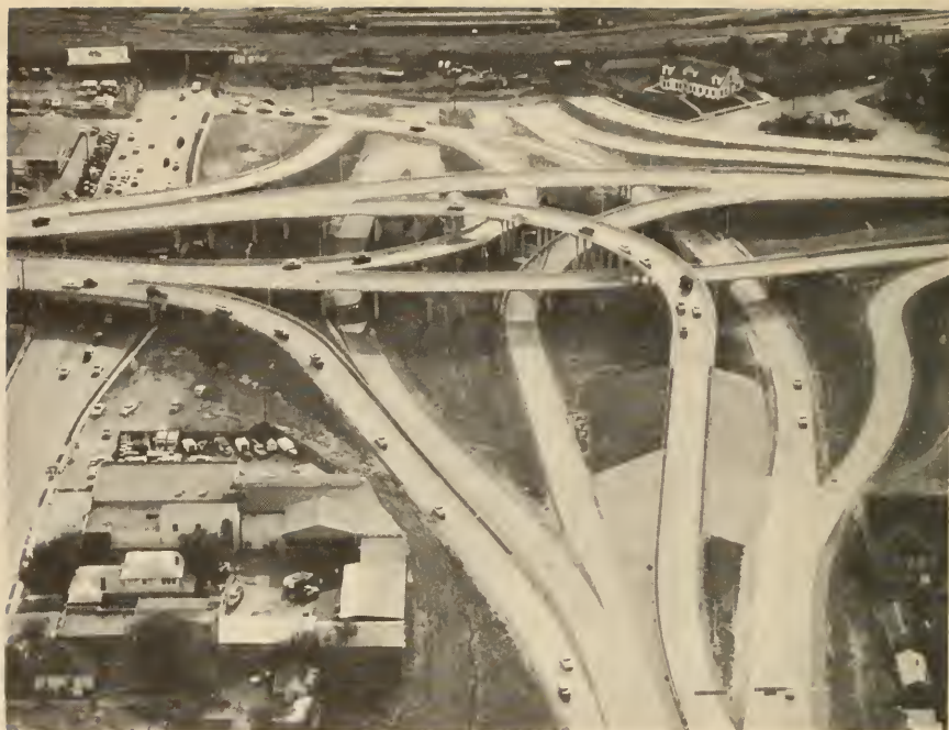
Texas Interstate Routes 35 and 20 intersect at this four-level interchange in Fort Worth.
