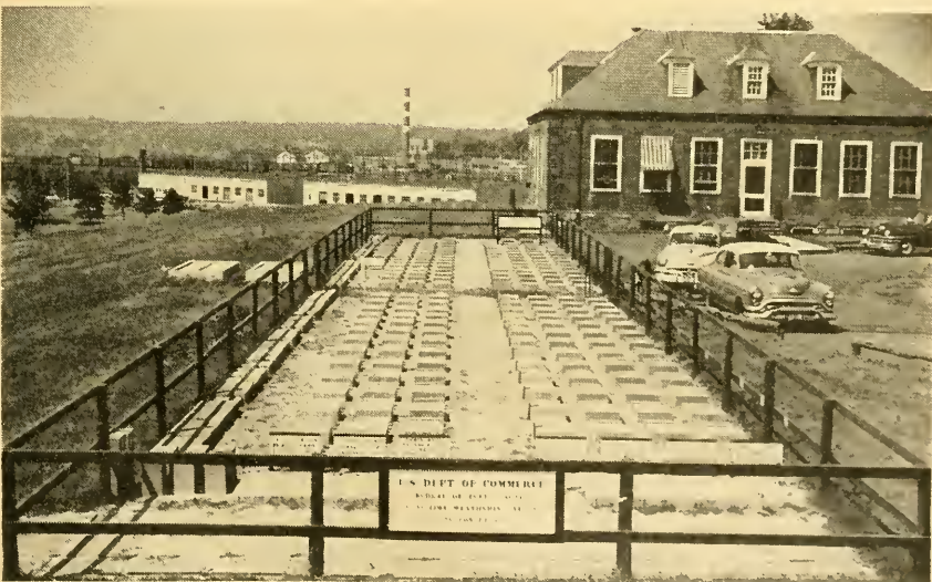
Long-time weathering tests of concrete at the Bureau of Public Roads laboratory.
