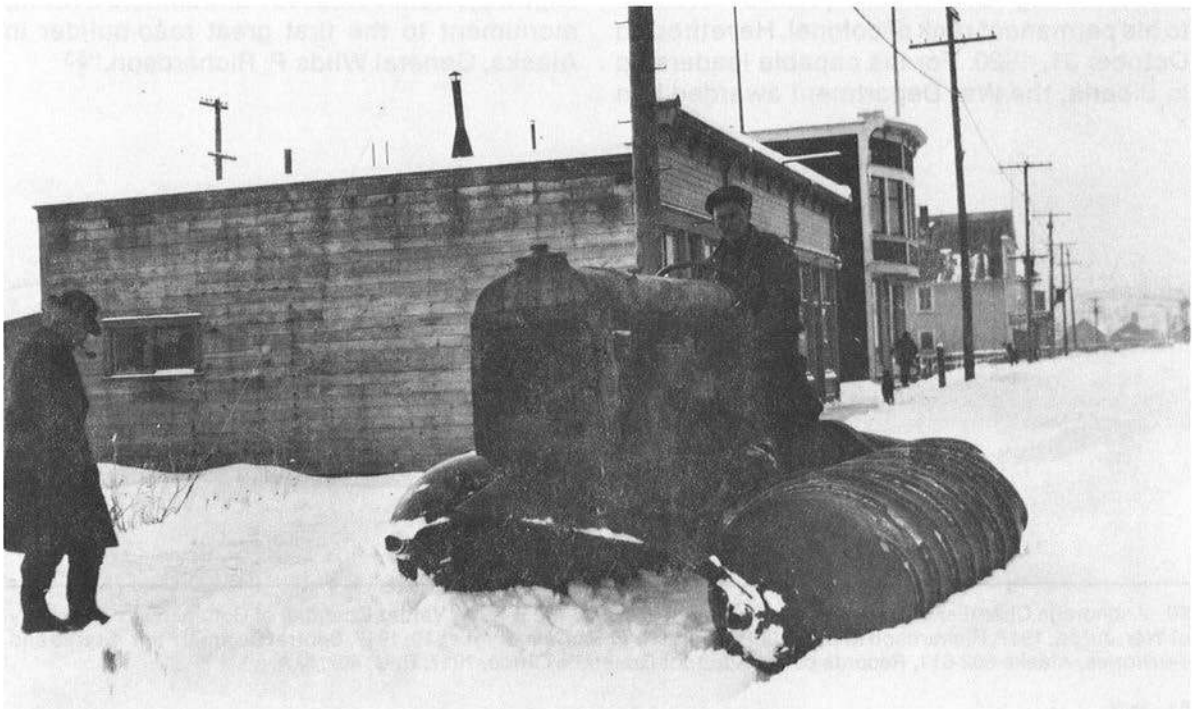
"Snow motor" with large revolving cylinders for propulsion, Valdez, November 27, 1929. Ray Huddleston Collection, UAF.
