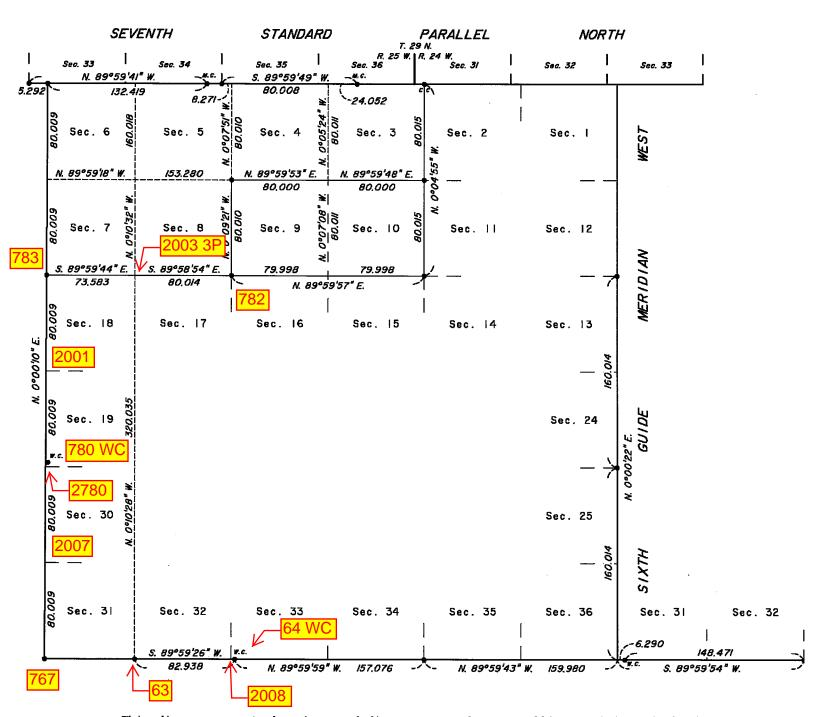
This diagram reports bearings and distances to the controlling positions defined by the relationship of identified recovered corners with the protracted lines shown on the official plat of survey accepted December 28, 1978.
