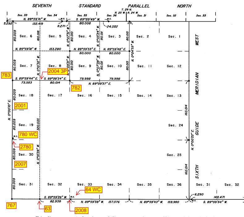
This diagram reports bearings and distances to the controlling positions defined by the relationship of identified recovered corners with the protracted lines shown on the official plat of survey accepted December 28, 1978.
