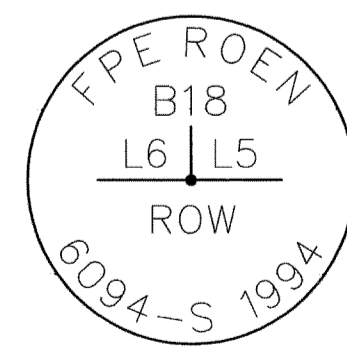
POINT 316 1.5" ALUMINUM CAP ON REBAR, FLUSH WITH GROUND.
