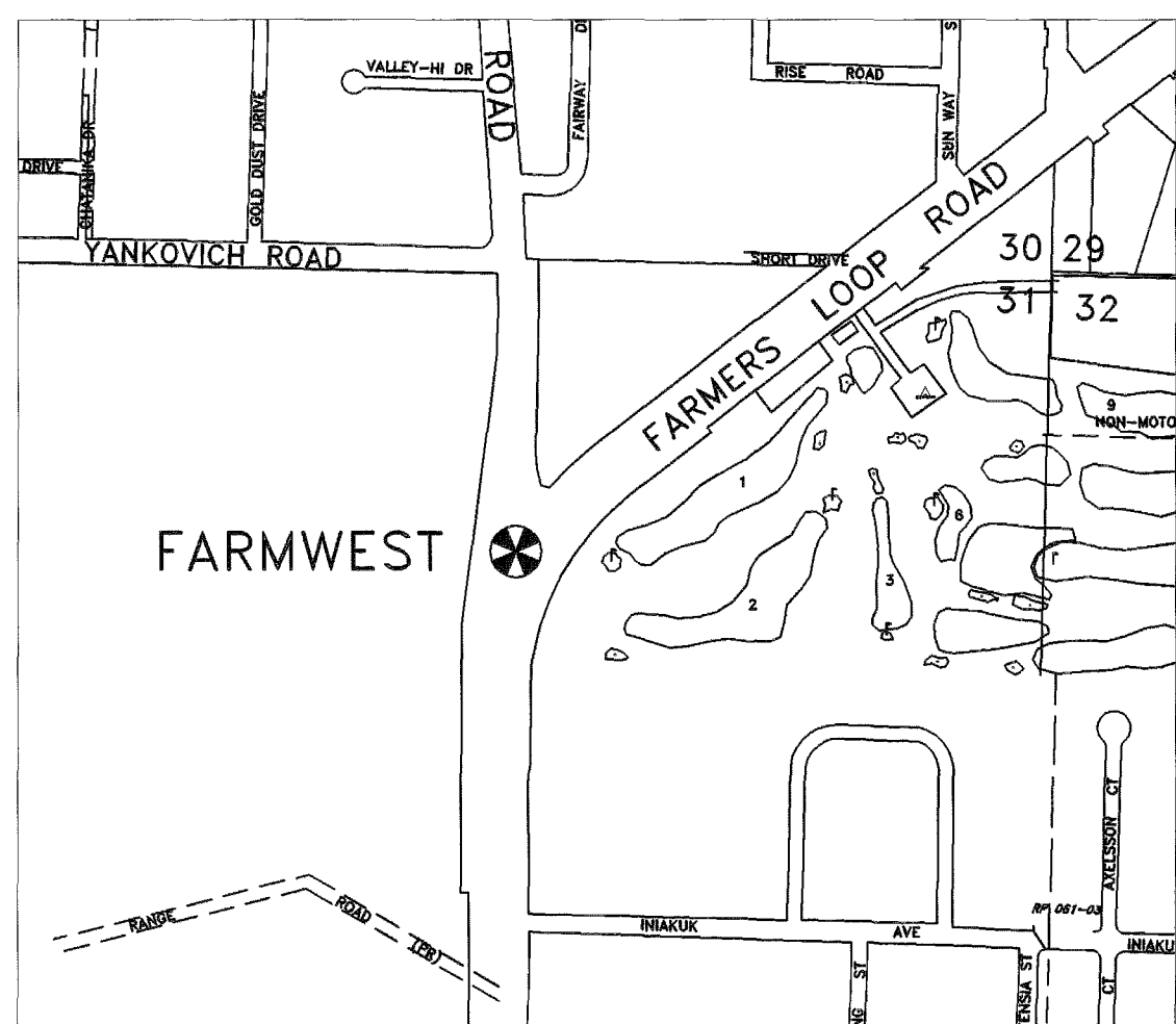
FARMWEST State of Alaska Primary Monument Set in Island Created by Ballaine Rd and Ballaine Acel Lane 5 Meters North of Farmers Loop Bike Path.
