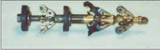
Figure 39. Example of a 3" pig used in the CANOL Pipeline. Courtesy George Lyle.
