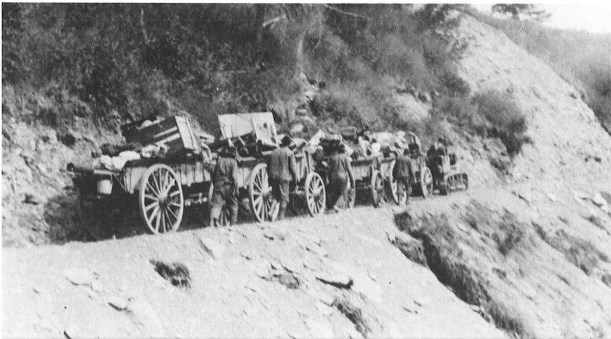
Wagons, formerly used with horses, being pulled by a caterpillar. The transition to motor power occurred in the late 1920s and early 1930s. Ray Huddleston Collection, UAF.
