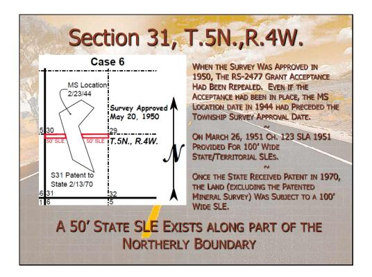
The Mineral Survey preceded and was not a part of the Rectangular System so no SLE can exist across it.
