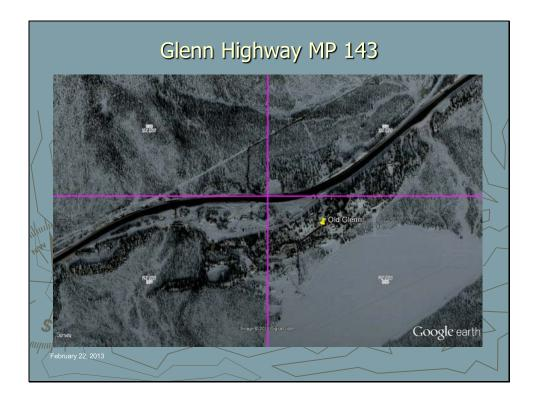
Current owner of USS 4824 requested evaluation of old ROW at MP 143. House may be in existing right of way. Old road realigned in 1975-6. Note old alignment to south in S1 & S6.
