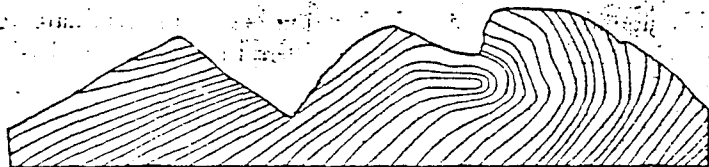
FIGURE 4.—Sketch showing overturned fold in Cantwell formation on East Fork of Toklat River. River bluff is 400 feet high.
