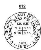
T3S R3E FM CORNER OF SECTIONS 9, 10, 16, & 15 FOUND 3 1/4" BRASS CAP ON 2 1/2" IRON POST, 0.5' ABOVE GRADE, GOOD CONDITION
