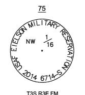
T3S R3E FM NORTH EAST 1/16 COR FOR SEC 16 CENTER NORTH 1/16 COR FOR SEC 16 NORTH WEST 1/16 COR FOR SEC 16 3 1/4" ALUMINUM CAP ON 2 1/2" ALUMINUM POST. 0.1' ABOVE GRADE SET CARSONITE WITNESS POSTS
