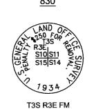
CORNER FOR SECS 10, 11, 15, & 14 FOUND 2 1/4" BRASS CAP ON 1 1/4" IRON PIPE, LAYING ON ITS SIDE AND BURIED, EXCAVATED AND RESET, 0.8' ABOVE GRADE, GOOD CONDITION
