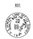
T3S R3E FM WCMC FOR SECTIONS 10 & 15 2 1/4" BRASS CAP ON 1 1/4" IRON POST, 0.7' ABOVE GRADE, GOOD CONDITION
