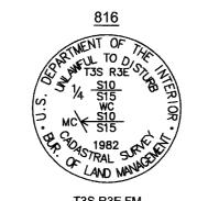
T3S R3E FM WCMC TO 1/4 COR FOR SECS 10 & 15 FOUND 3 1/2" BRASS CAP ON 2 1/2" IRON POST, 0.3' ABOVE GRADE GOOD CONDITION
