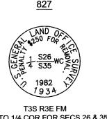
T3S R3E FM WC TO 1/4 COR FOR SECS 26 & 35 CORNER FOR SECS 22, 23, 27, & 26 FOUND FOUND 2 1/2" BRASS CAP ON 2" IRON PIPE, 2 1/4" BRASS CAP ON 1 1/4" IRON POST, 1.1' ABOVE GRADE, 0.4' ABOVE GRADE, GOOD CONDITION GOOD CONDITION
