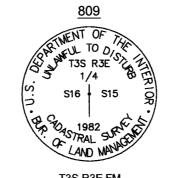
T3S R3E FM 1/4 CORNER FOR SECTIONS 16 & 15 FOUND 3 1/2" BRASS CAP ON 2 1/2" IRON POST, IN MON CASE, 1.0' BELOW LIP OF ASPHALT ROADWAY GOOD CONDITION
