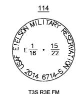
T3S R3E FM EAST 1/16 COR FOR SECS 15 & 22 3 1/4" ALUMINUM CAP ON 2 1/2" ALUMINUM POST. 0.5' ABOVE GRADE SET CARSONITE WITNESS POSTS
