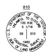
SOUTH 1/16 COR FOR SECS 9 & 10 3 1/2" BRASS CAP ON 2 1/2" IRON POST, 0.5' ABOVE GRADE GOOD CONDITION
