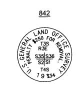
T3S/T4S R3E FM CORNER FOR SECS 35, 36, 2, & 1 FOUND 2 1/2" BRASS CAP ON 2" IRON PIPE, 0.7' ABOVE GRADE, GOOD CONDITION
