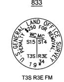
WCMC FOR SECTIONS 15 & 14 FOUND 2 1/4" BRASS CAP ON 1 1/4" IRON POST, BENT AND LEANING NORTHEAST, STRAITENED TO ORIGINAL POSITION, 0.8' ABOVE GRADE, GOOD CONDITION
