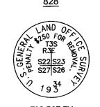
T3S R3E FM CORNER FOR SECS 22, 23, 27, & 26 FOUND 2 1/2" BRASS CAP ON 2" IRON PIPE, 0.4' ABOVE GRADE, GOOD CONDITION
