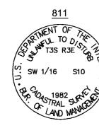
T3S R3E FM SOUTH WEST 1/16 COR OF SEC 10 FOUND 3 1/2" BRASS CAP ON 2 1/2" IRON POST, 0.1' ABOVE GRADE GOOD CONDITION
