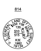
T3S R3E FM WCMC FOR SECTIONS 10 & 15 FOUND 2 1/4" BRASS CAP ON 1 1/4" IRON POST, 1.0' ABOVE GRADE, GOOD CONDITION
