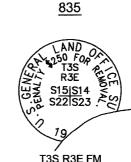
T3S R3E FM CORNER FOR SECS 15, 14, 22, & 23 FOUND 2 1/2" BRASS CAP ON 2" IRON POST, 0.4' ABOVE GRADE, 5" ALDER GROWING AROUND EDGE OF MONUMENT, GOOD CONDITION
