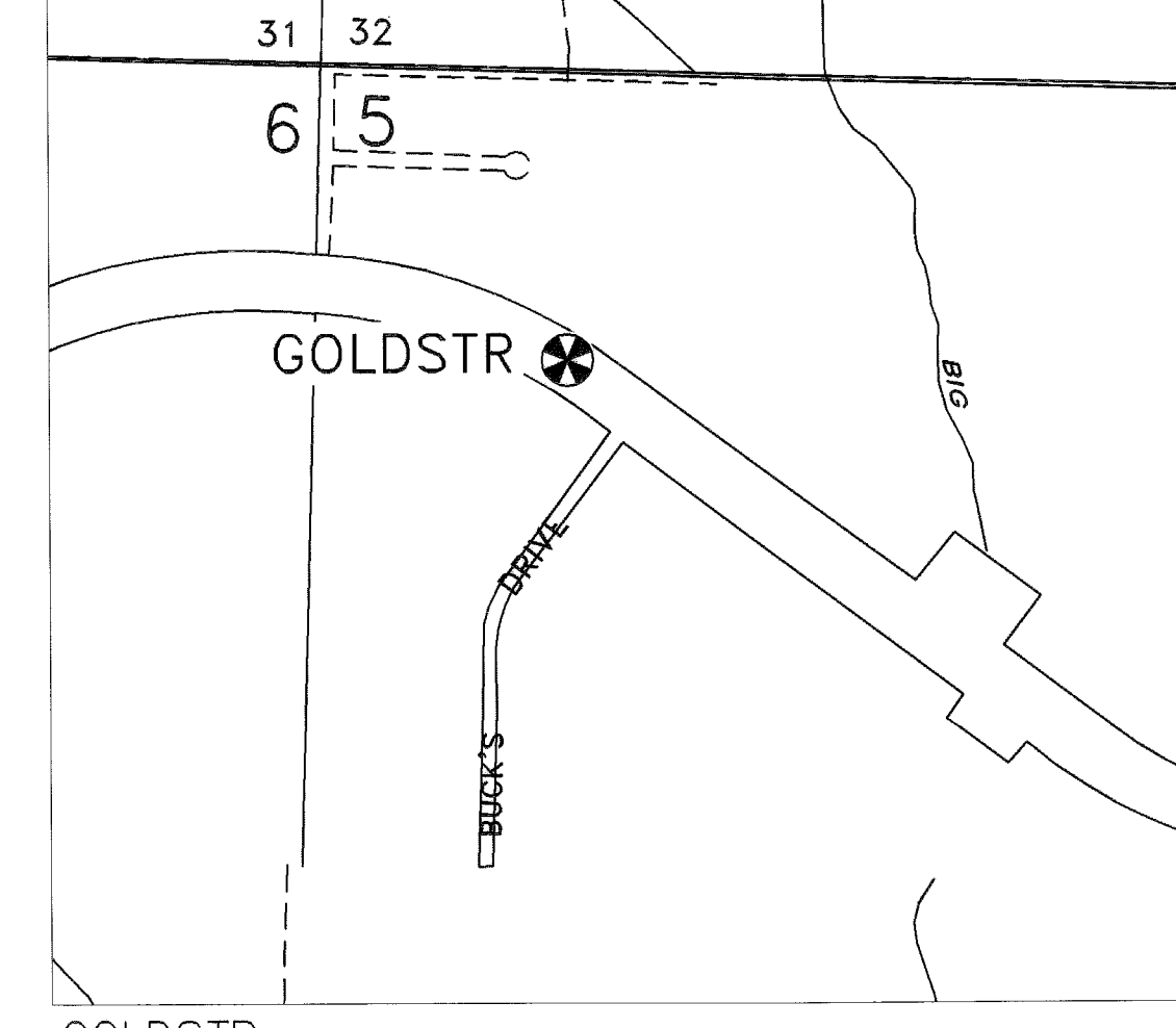
GOLDSTR State of Alaska Primary Monument Set 11 Meters East of Easterly End of Turnout and 5 Meters North of the Shoulder of Goldstream Rd. and 76 Meters West of Buck Drive on Goldstream Rd.
