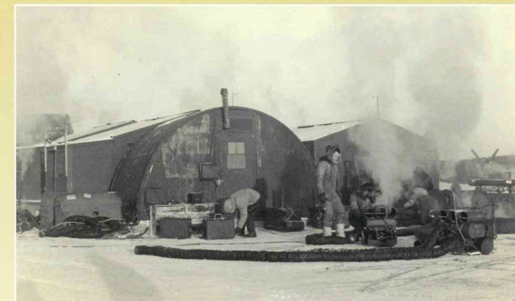
Cold Weather Test Detachment ground equipment test area, east side of Hangar One. Note C-13 battery carts and Herman-Nelson heaters. Temperature -35°F. AAF photo ca. 1944, courtesy Russ Sackett.
