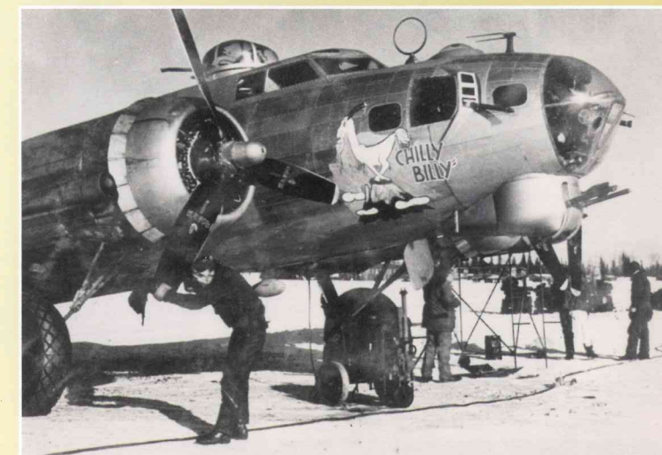
Chilly Billy, a B-17G, receives cold weather preparation for the arctic environment. Courtesy Randy Acord.
