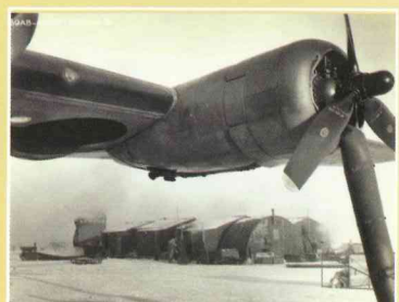
B-24 with engine heater (duct) at 35°F below. Courtesy Randy Acord.
