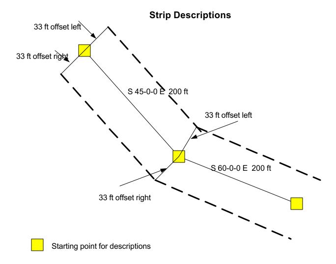
Strip descriptions - description of a centerline with an offset on either side. Ccan also be a radial description with a center point and a distance or radius around the point. Sometimes stationing is provided along the line with the offset along the stationing. Problems include:
