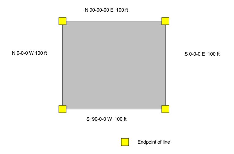
Metes descriptions - perimeter descriptions with a direction of travel described by a series of measurements. Problems include:
